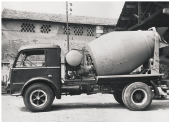
◀ 1958 Autobetoniera 400 azionata da motore ausiliario "400" model truck-mixer driven by auxiliary engine
