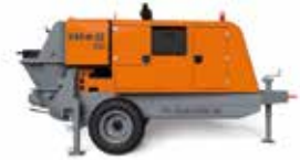
PC506 Max theoretical output: 52 m 3 /h Max pressure on concrete: 41 bar
