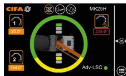
LSC LIGHT STABILITY CONTROL (according to EN 12001:2012)
