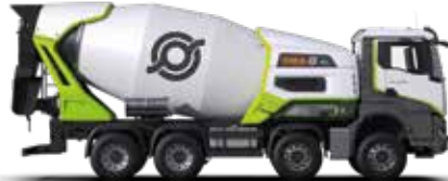
BEE E9 MIXER Nominal capacity: 9 m 3
