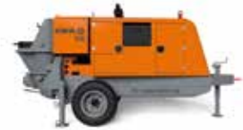
PC607 Max theoretical output: 60 m 3 /h Max pressure on concrete: 67 bar
