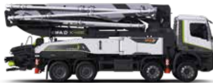
BEE K42E TRUCK PUMP Boom height: 41,1 m Boom sections: 5
