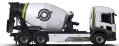
BEE SLE7 MIXER Nominal capacity: 7 m 3
