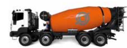
HD/HDA Nominal capacity: 7-8-9-10-12-15 m 3 Available with Auxiliary Engine
