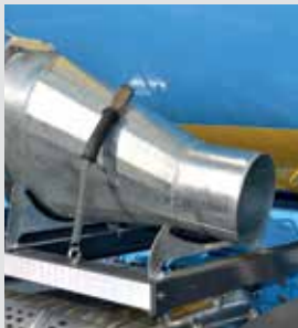
Cone-shaped chute with end diameter 200 mm.
