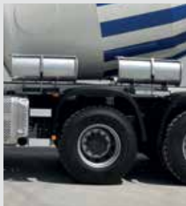
Additional two discharge chute pieces with supports.
