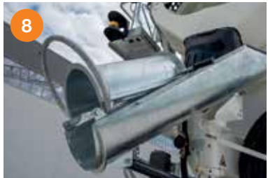
Fold over chute (1500 mm) with anti-shear device.
