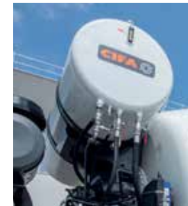
Module with 1200 litre water tank and integrated oil tank
