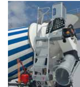
Basic equipment compliant with the EN 12609 standard with rear underrun and cyclist protection bars, rear camera, LED rear light, anti-shear system on the discharge chute and platform on the loading hopper
