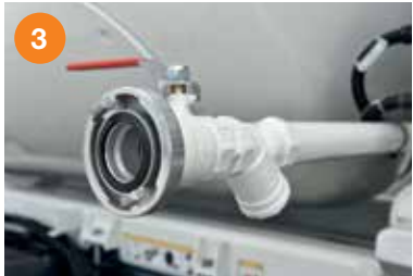
Quick-fit water connector on both sides of the mixer.
