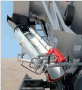
"SL45" 4.5 m hydraulic discharge chute with 3 extensions.
