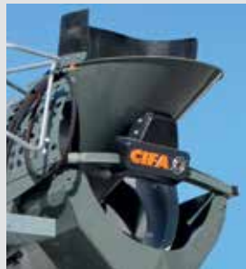
Rubber sleeve on the loading hopper.
