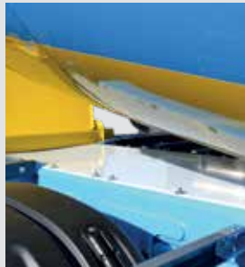
Protection between frame and drum.
