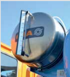
Aluminium pressurised water tank (capacity 600 litres).
