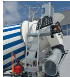
Basic equipment compliant with the EN 12609 standard with rear underrun and cyclist protection bars, rear camera, LED rear light, anti-shear system on the discharge chute and platform on the loading hopper
