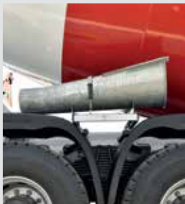
Cone-shaped chute for "SL45".
