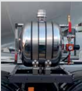
Additive pressurised tank (50 litres) made of stainless steel.
