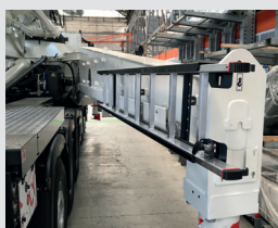
Ladder to fuel tank access
